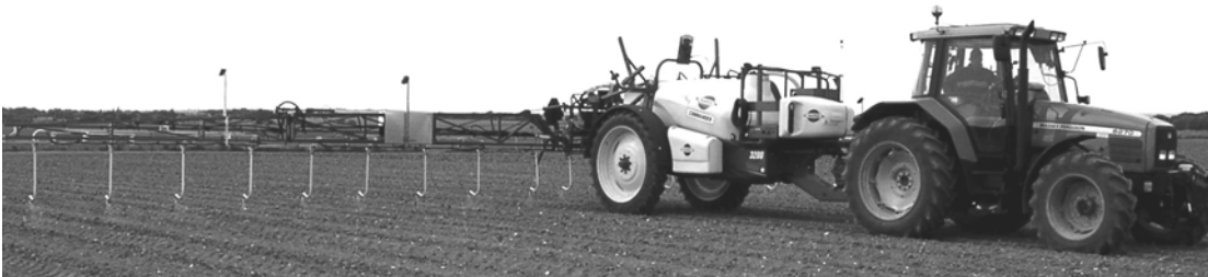
Figure 3 Experimental vision guided band sprayer spanning 20m with one fixed and four independently controlled 4m wide sections
