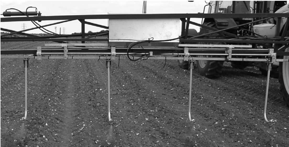
Fig. 4. Drop legs with flat fan nozzles viewed from behind and aligned over crop rows
