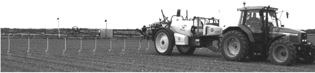
Fig.3. Experimental vision guided band sprayer spanning 20m with one fixed and four independently controlled 4m wide sections
