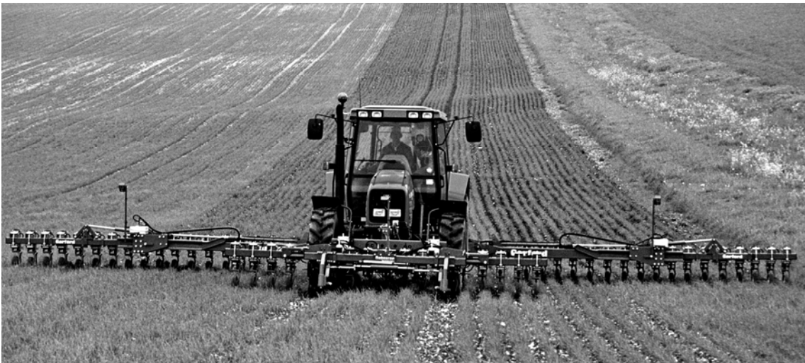
Fig. 1. Experimental vision guided hoe spanning 12m with three independently controlled 4m wide sections
