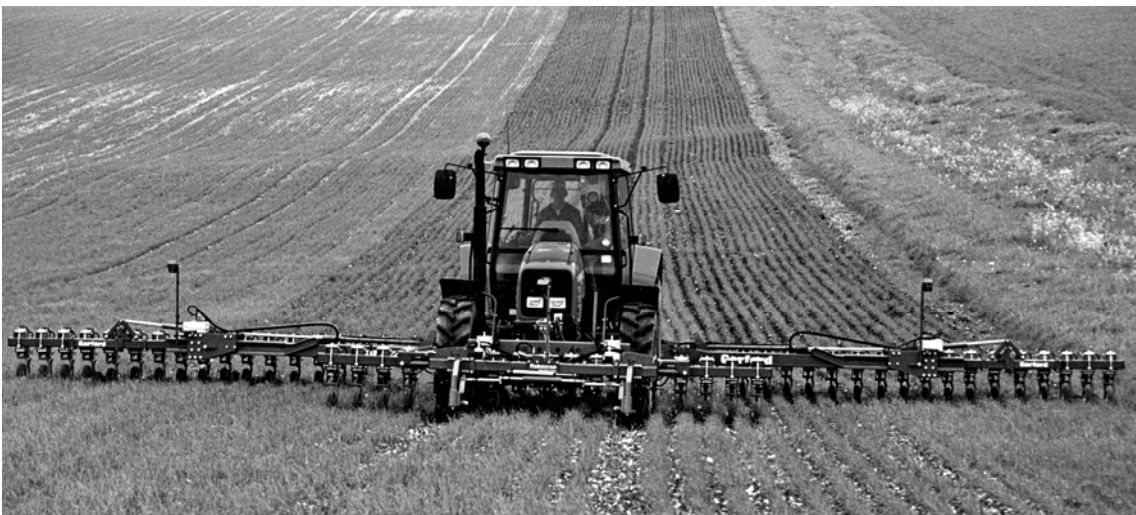
Figure 1 Experimental vision guided hoe spanning 12m with three independently controlled 4m wide sections.
