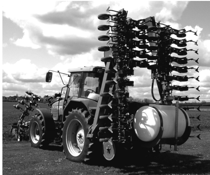
Figure 2 Experimental hoe folded for road transport with band spraying tank fitted
